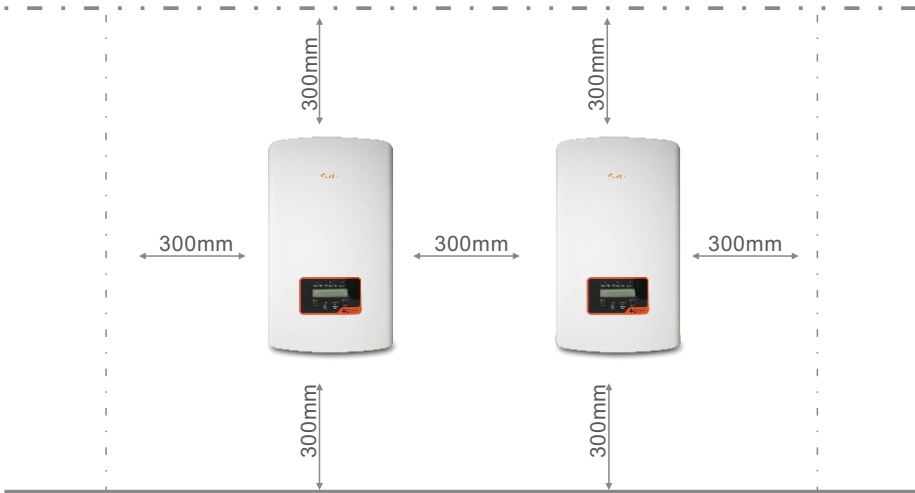
▲ Figure 4.2 Inverter Mounting clearance
