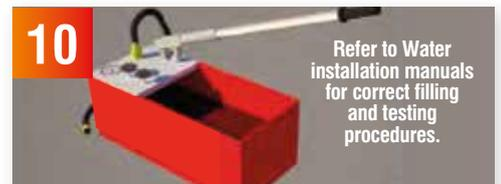
10 Refer to Water installation manuals for correct filling and testing procedures. Upon completion of the underfloor heating pipe circuits - ensure all pipe work is pressured tested ( conforming to BS EN 1264). The mixing valve temperature should not be set above 55 degrees Celsius for floating floor or solid floor systems.
