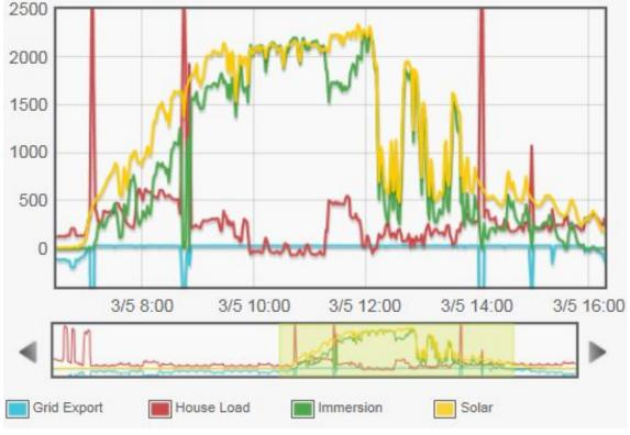
Even on days when the sun and the house load is less steady the blue line still shows tiny export showing how fast the device reacts to changes in conditions.
